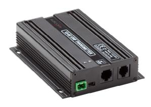
Configuration of the transmitter is performed via the USB port or the serial port using an intuitive Salcom programming application which allows for the setting of all operational parameters.
